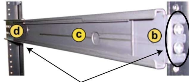
Secure with 2 screws to both front and rear posts. After you have secured the slide rail fingers to the rack posts, tighten the 2 screws used to attach the slide rail **b** to the end bracket **d**.
