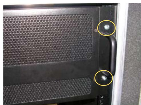
Use 2 Panhead screws, on each side, to secure the chassis to the rack as shown.
