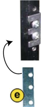
If your rack has holes too large for the screws, you can use the Bar Nut **e** to secure your mounting by inserting the Panhead screw through the rack hole and screwing it into the Bar Nut on the reverse side of the rack post, as shown. Notice that the holes on the Bar Nut are spaced unevenly to accommodate different racks.
