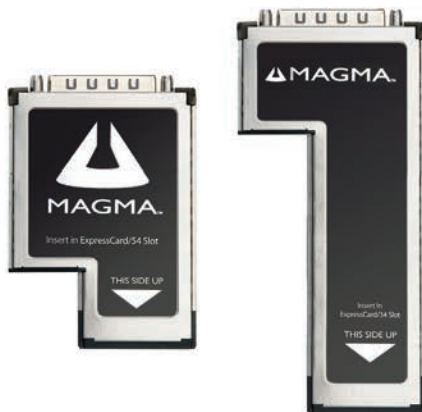
Easy expansion solution for laptops with optional Magma ExpressCards for connection to laptops.
